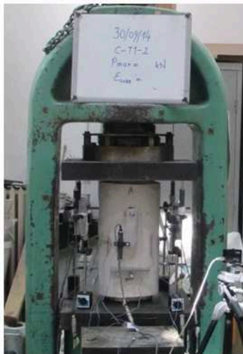
Figure 2. Test set-up and stress-strain relationships obtained from uniaxial compression tests
